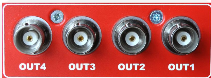
Figure 12: output BNC connectors (default 2-channel configuration)
