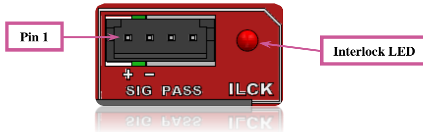
Figure 6: Interlock connector of the board
