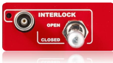
Figure 7: Interlock of the HV-ADAPTOS system crate
