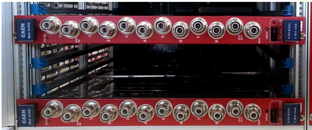
Figure 9: A1522 high-voltage boards installation
