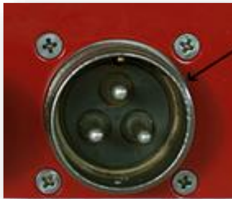
Figure 5: AC Mains mating connections
