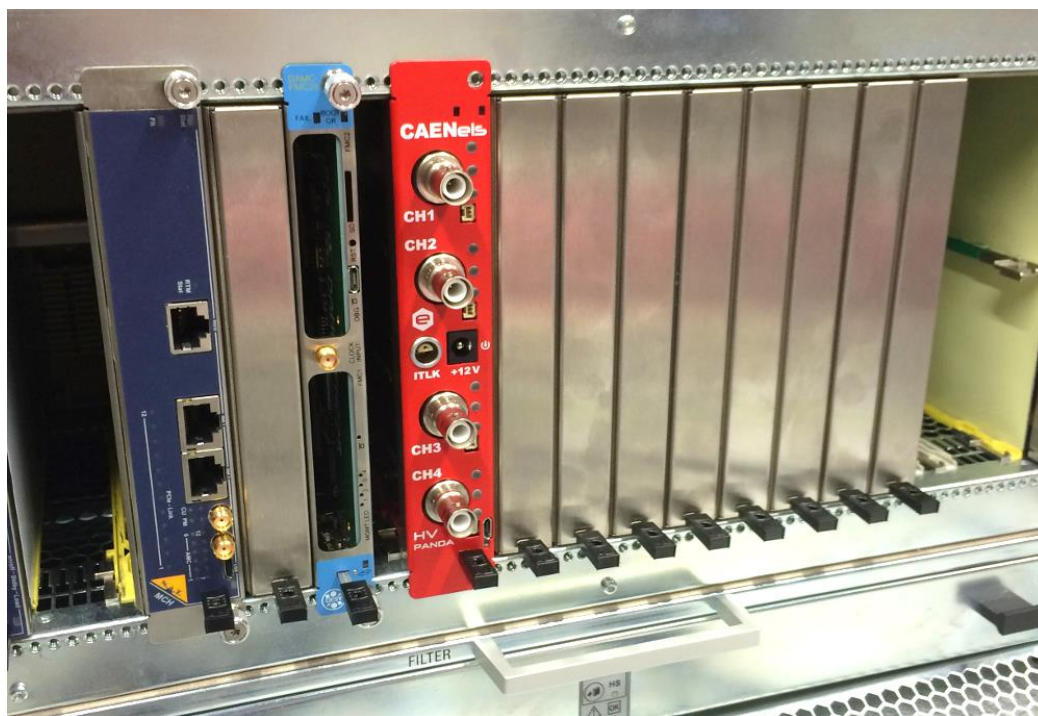
Figure 2.2 : AMC fully inserted in the MTCA chassis
