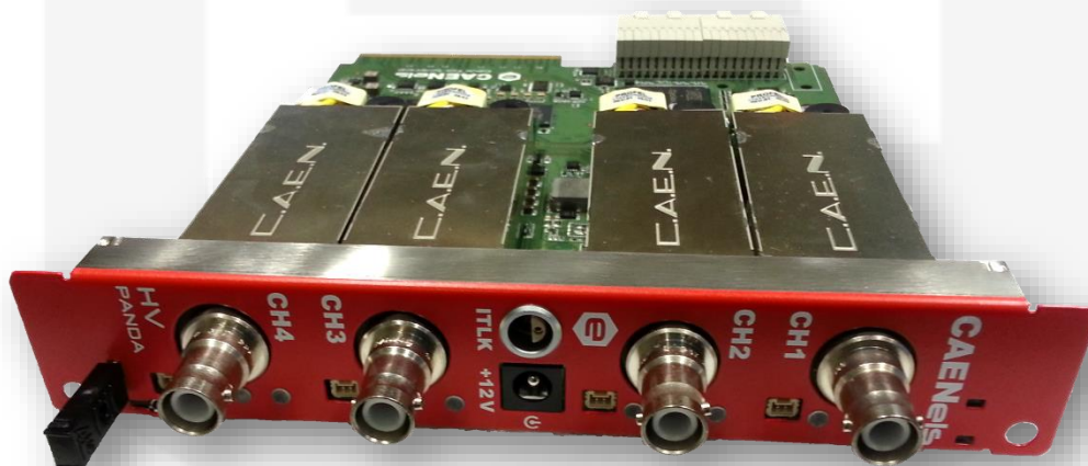
Figure 3: AMC HV-PANDA front view
