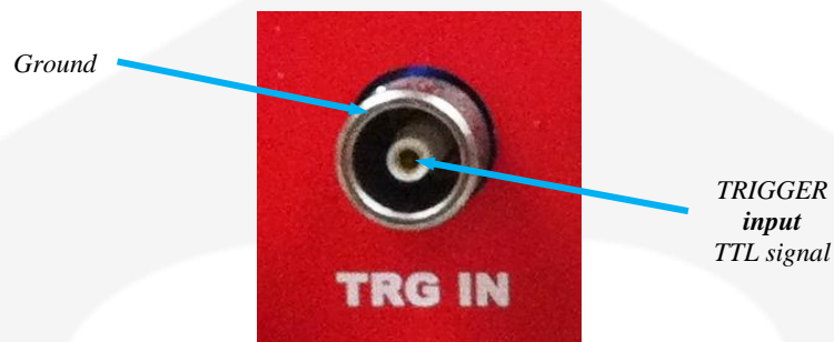
Figure 5 – Trigger input connector
