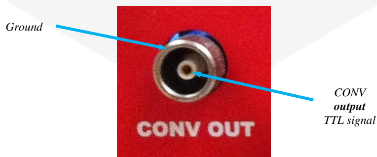
Figure 6 – CONV output connector
