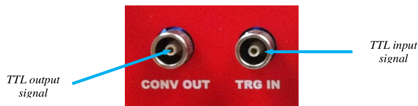
Figure 4 - I/O Interface Connector
