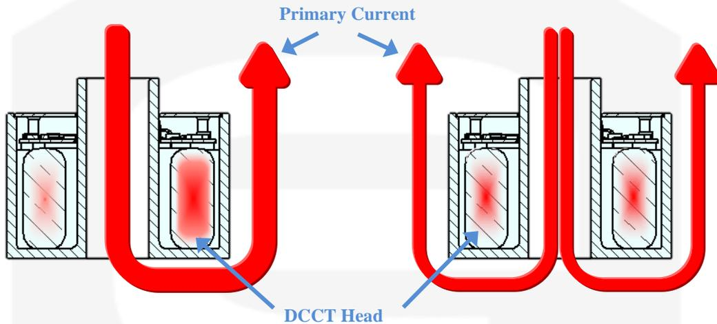
**Figure 10:** primary current path; non-recommended layout (left) and recommended layout (right)
