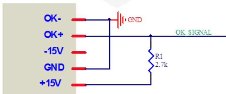
**Figure 5:** OUT OK signals connections using the +15V and the GND pins
