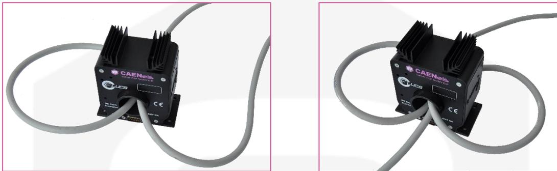
**Figure 11:** primary full-scale current scaled by a factor 2 (2 primary turns - left) and scaled by 3 (3 primary turns - right)
