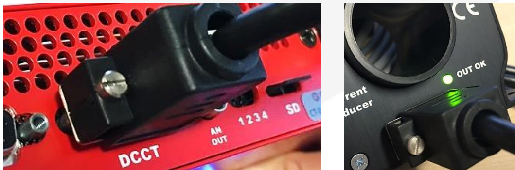
Figure 5: Connection of the DCCT cable
