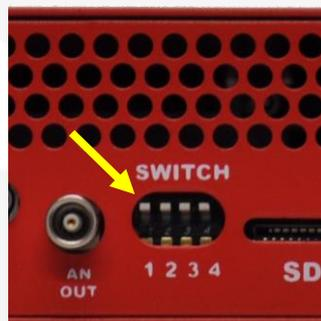
**Figure 13:** SWITCH position for update firmware.
