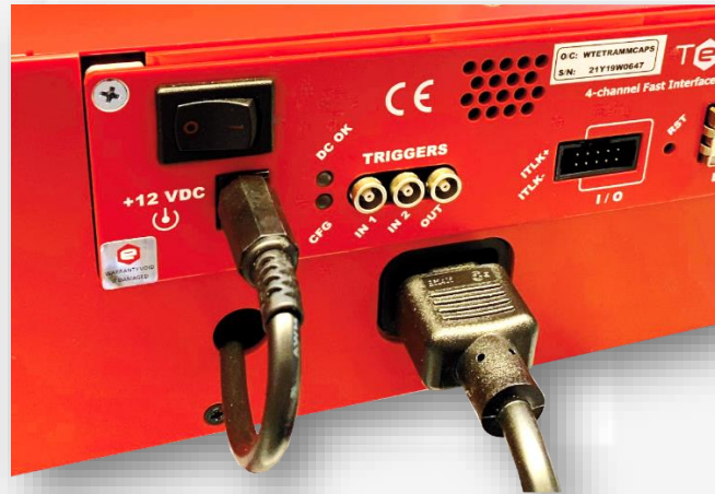
Figure 30: power supply connections
