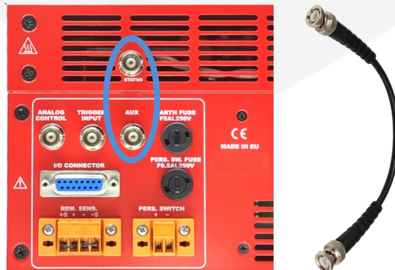
Figure 2: “Status cable” connection
