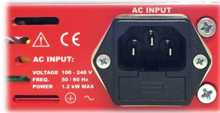
Figure 14: AC Power Line input socket
