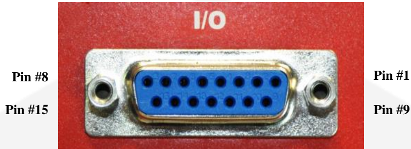
Figure 5: I/O Connector
