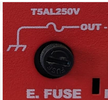
Figure 28: Earth fuse housing.
