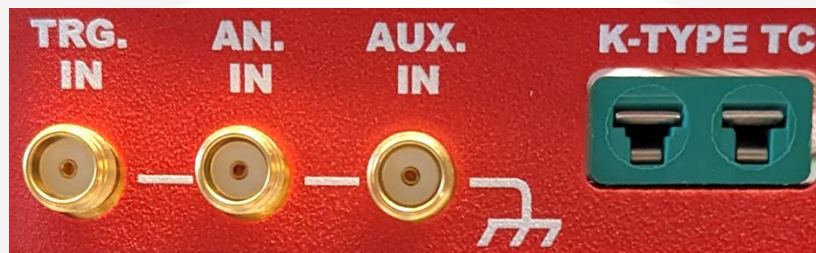
Figure 20: SDA jack input connectors and K-type for thermocouple.
