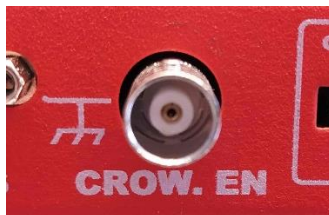
Figure 29: Crow-bar enable connector on the rear panel.
