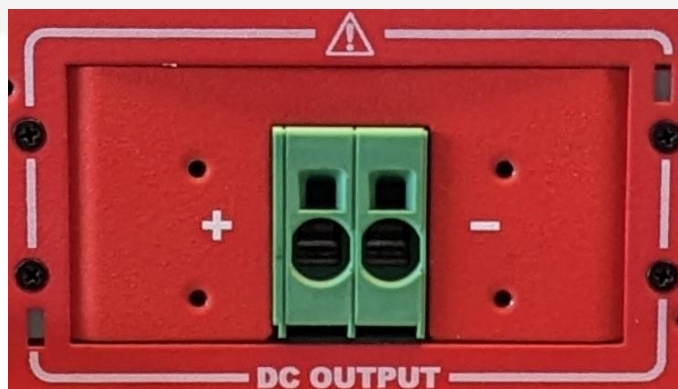
Figure 24: Output Connector for High-Voltage models, without cover.
