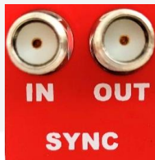
Figure 19: SYNC IN and SYNC OUT connectors
