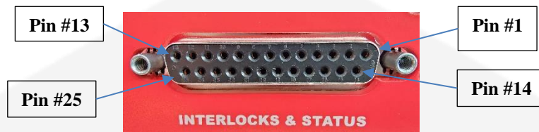
Figure 13: Interlock and Signal Status Connector
