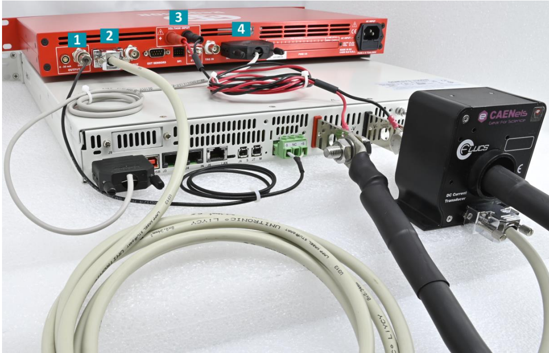
Figure 21: Setup of the Regul8OR/external power supply system (e.g. TDK-LAMBDA of the GENESIS+ family). Note the presence of the DCCT for the current sensing on the output terminals of the power supply.
