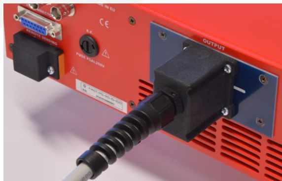
Figure 22: Install the safety cover
