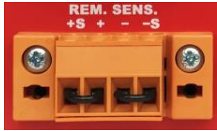
Figure 6: Factory mating Remote Sensing connector
