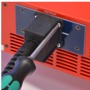
Figure 21: Connect the wire to the output connector
