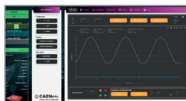
Embedded Web-Server with AWG and OSCILLOSCOPE
