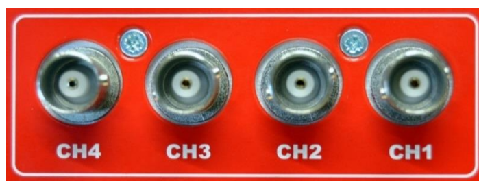
Figure 8: BNC input connectors
