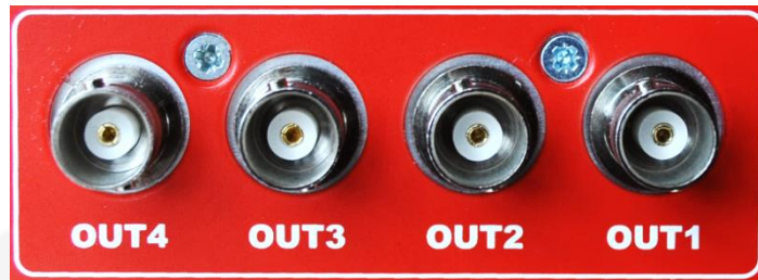
Figure 10: PreDAC BNC output connectors
