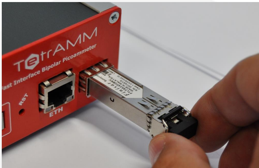
Figure 11: Connection of the SFP optic transceiver into its slot
