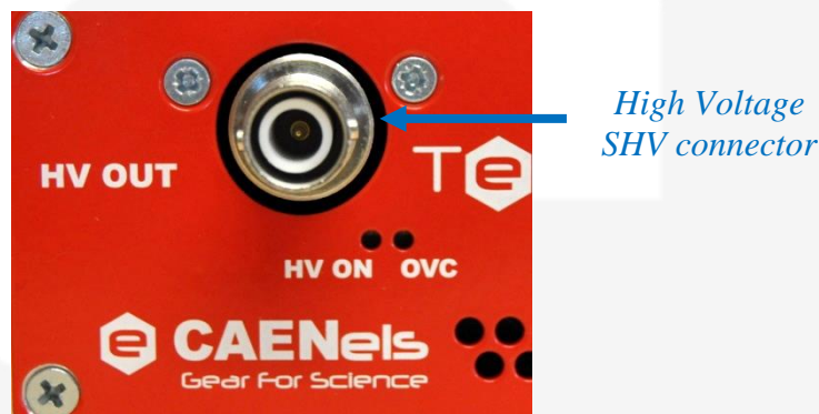
Figure 9: High Voltage SHV connector
