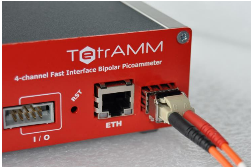
Figure 12: SFP connection
