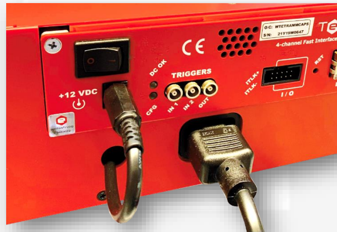
Figure 30: power supply connections
