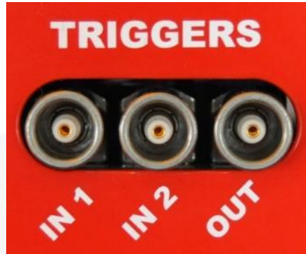
Figure 11: “Triggers” connectors on rear panel
