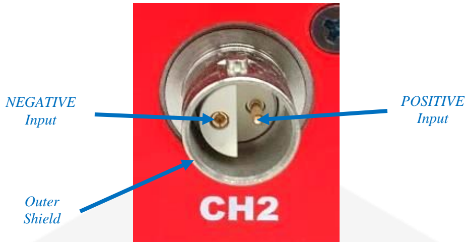
Figure 16: Pinout for the TWIN BNC connector
