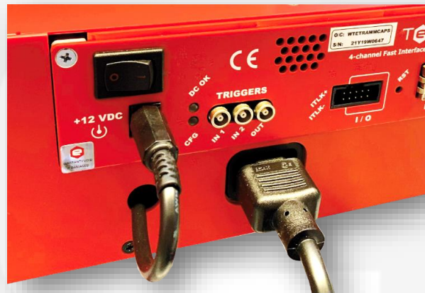
Figure 31: power supply connections
