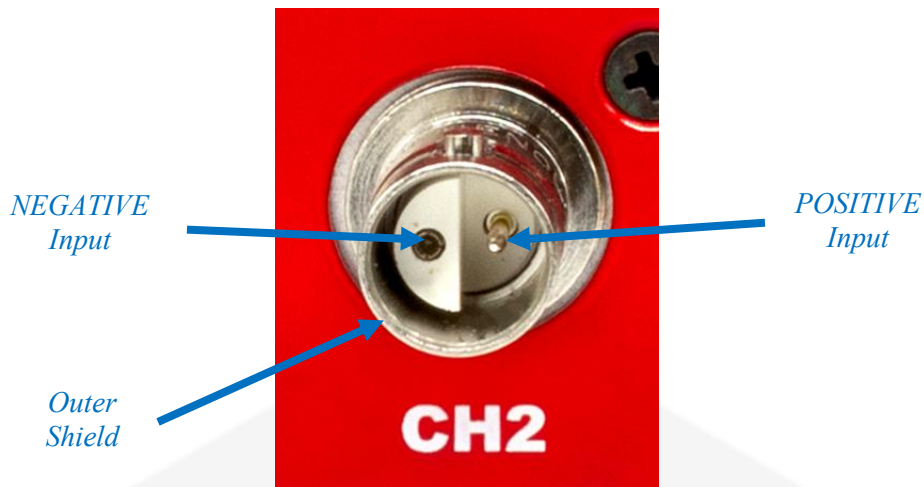
Figure 16: Pinout for the TWIN BNC connector
