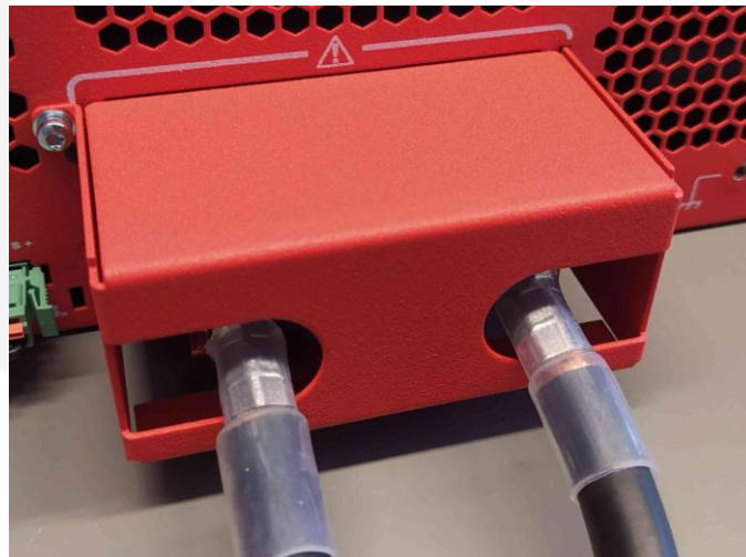
Figure 23: Output terminals for High-Current models with cover and load connected.
