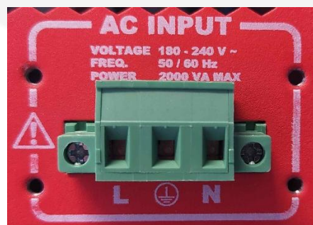
Figure 5: AC Power Line input with terminal block.
