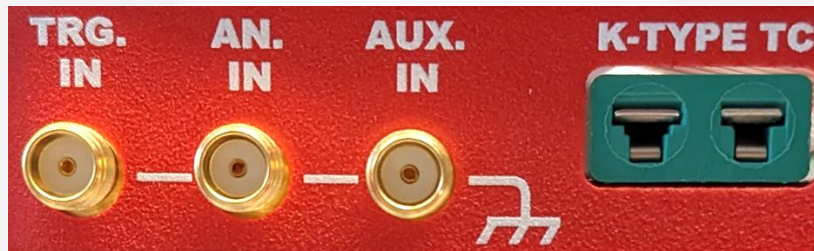
Figure 20: SDA jack input connectors and K-type for thermocouple.
