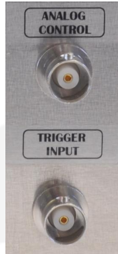
Figure 8: Trigger and analog input connectors
