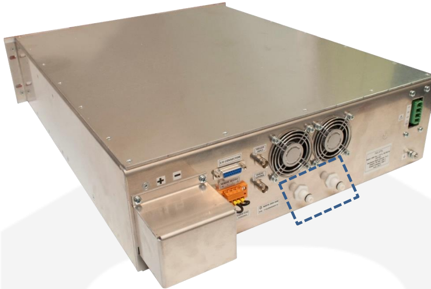
Figure 3: Water cooled NGPS rear view. Plugs for the connection to the hydraulic system are highlighted
