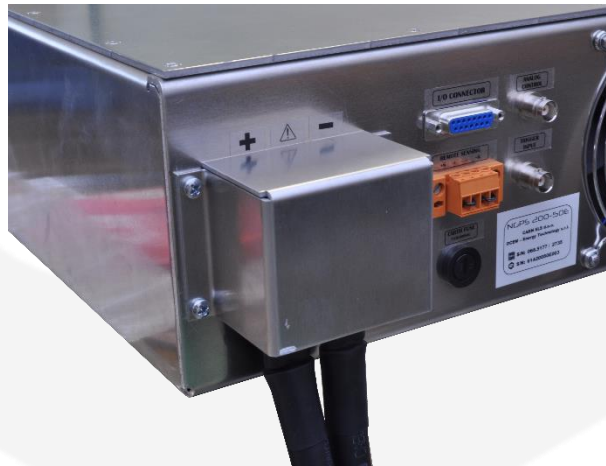
Figure 19: Metallic protective cover on the output terminal connections
