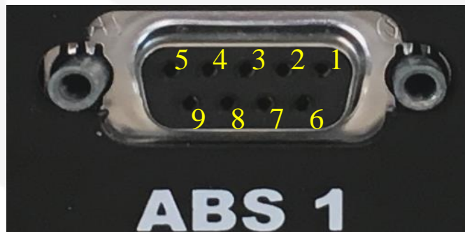
Figure 8: Absolute encoder connector
