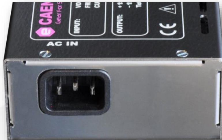
Figure 16: AC Line input connector
