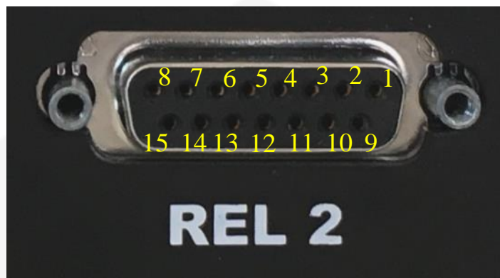
Figure 9: Relative encoder connector
