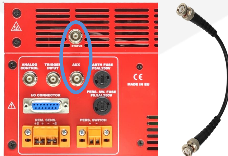
Figure 2: “Status cable” connection
