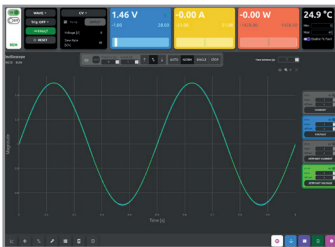
Embedded Web-Server with AWG and OSCILLOSCOPE
