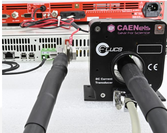
Figure 22: Orientation of the DCCT transducer for the output current sensing of the power supply.
