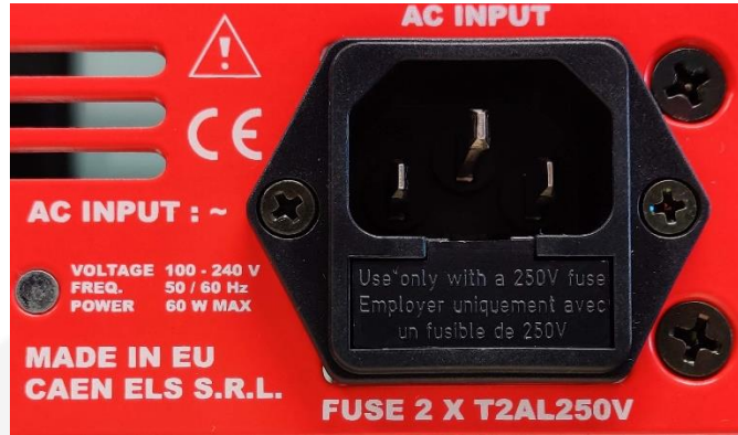
Figure 12: AC Power Line input socket
