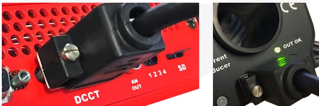
Figure 5: Connection of the DCCT cable
