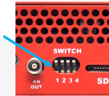
Figure 17: SWITCH position for update firmware
