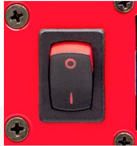
Figure 6: Power switch ON position
