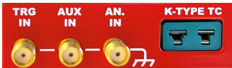
Figure 22: SMA jack input connectors and Type K IEC for thermocouple.
