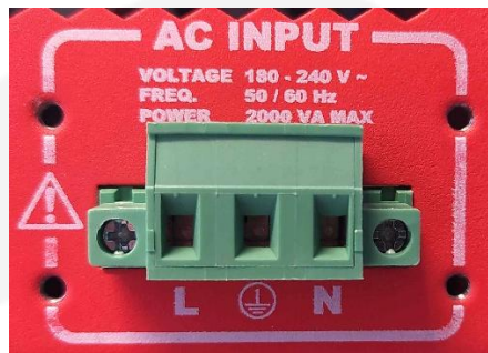
Figure 5: AC Power Line input with terminal block.
