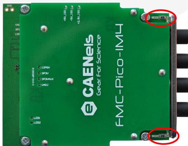
Figure 10: Jumpers for connecting the bezel to the input connectors
