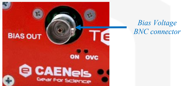
Figure 14: Bias Voltage BNC connector
