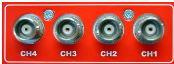
Figure 13: BNC input connectors
