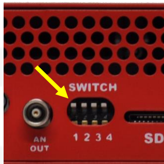
Figure 3.1: SWITCH position for update firmware.
