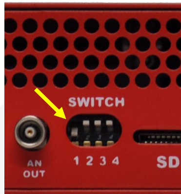
Figure 3.4: SWITCH position for normal use.
