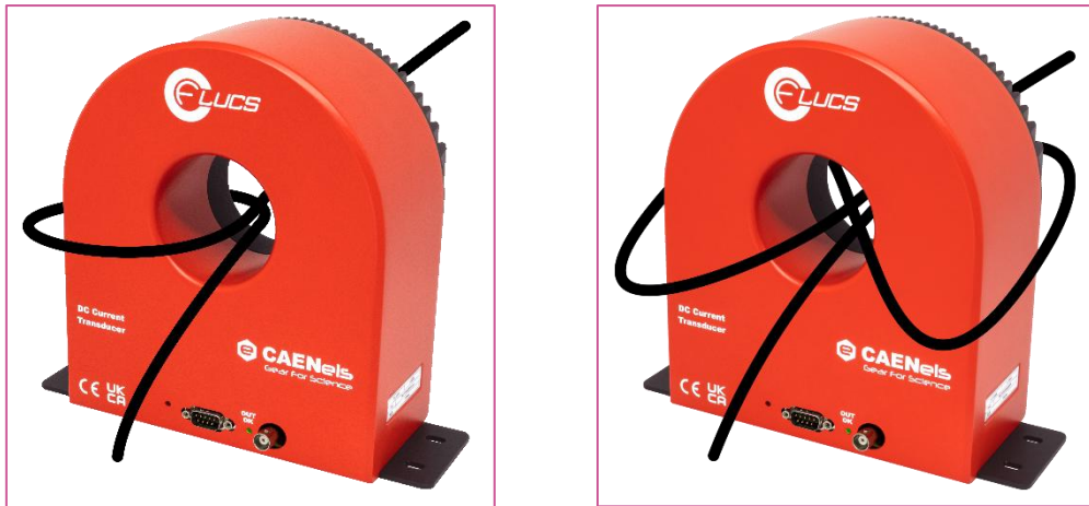
Figure 12: primary full-scale current scaled by a factor 2 (2 primary turns - left) and scaled by 3 (3 primary turns - right)
